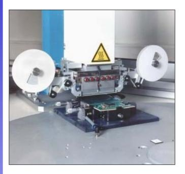
The Interposer Module is used in the Heat-Seal system to protect the products during the bonding process and to improve the bond strength. The Module uses silicon tape and is attached to the Quick Connect Block Module. Due to separated left and right submodules it's independent of Thermode length! As an additional feature, the small black guiding wheels offers spring tension control for the silicone tape itself. The Interposer Module can be mounted on most Unitek Eapro Heat-Seal bonding systems.
