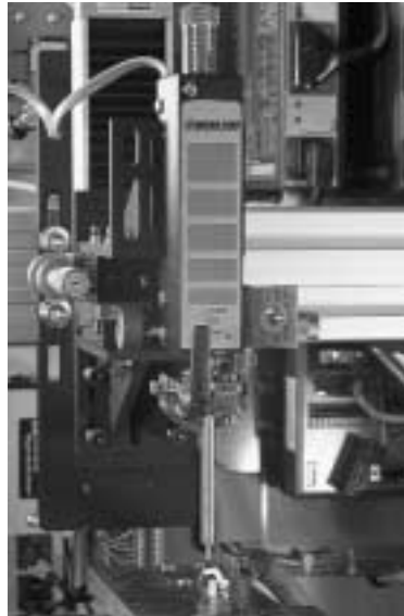
Model 400M Opposed electrode configuration for in-line welding.
