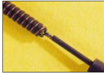
Cellular phone antenna assembly
