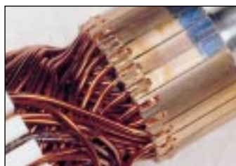
Slotted motor armature fusing
