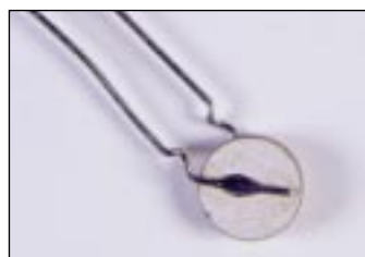
Piezo electrical device
